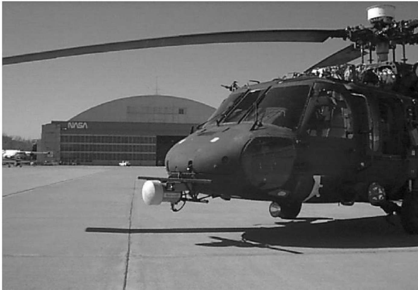
FIGURE 14.5 Honeywell 35-GHz biphase modulated CW obstacle avoidance radar [ http://ccf.arc.nasa.gov/dx/basket/pix/RASCAL.jpg ] (Photo—Dominic Hart).
